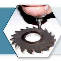
The ultrasonic (UCI) probe allows for hardness measurements of products in grooves and gear teeth due to its small contact area. Additionally, a special nozzle can be used to accurately measure the hardness of curved surfaces and wires.
