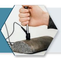
The dynamic (Leeb) measurement method is less demanding on material uniformity and surface roughness. This allows users to measure the hardness of a wide range of alloys and test products without preparing the testing surface.
